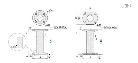
Prefabricated pipes for gas transportation
