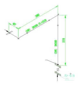
Connection Of Spiral Steel Pipeline And ASTM Socket Flange
